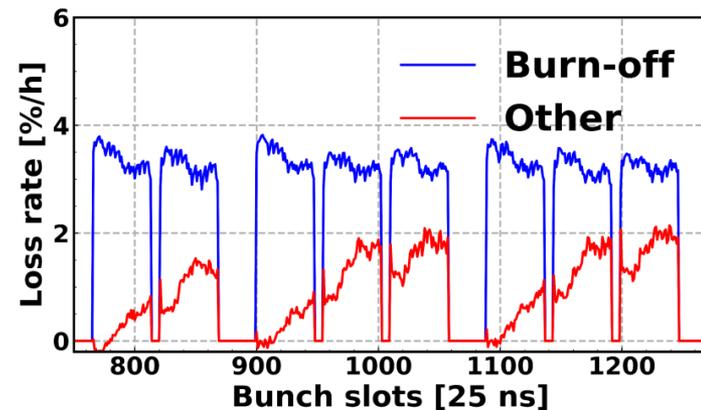
The bunch-by-bunch pattern of the **losses resembles the e-cloud buildup** simulations of the Inner Triplet quadrupoles.
