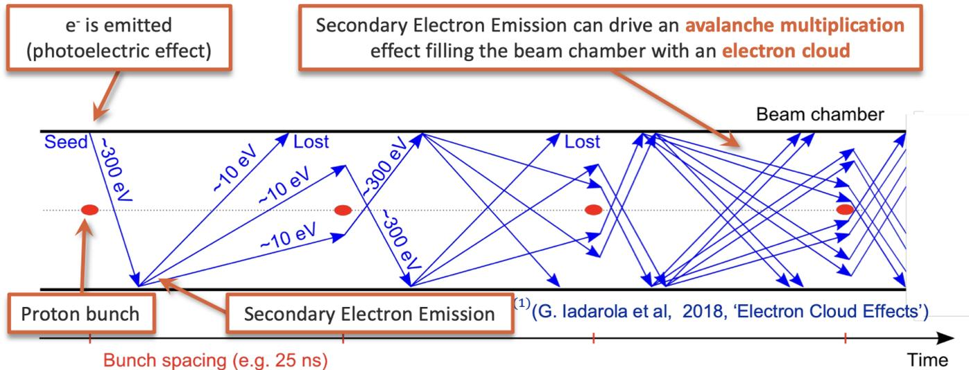
1. Electrons are introduced into the beam chamber (residual gas ionization / synchr. rad. + photoelectric effect)
