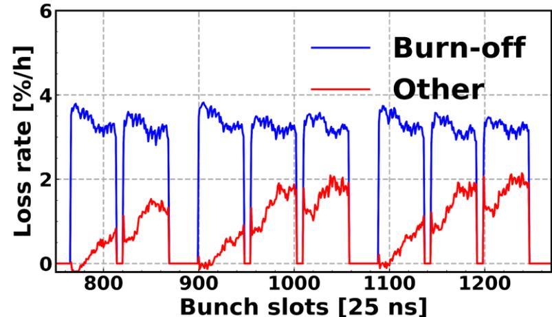
Universal characteristic of e-cloud to grow from the head to the tail of a beam.
