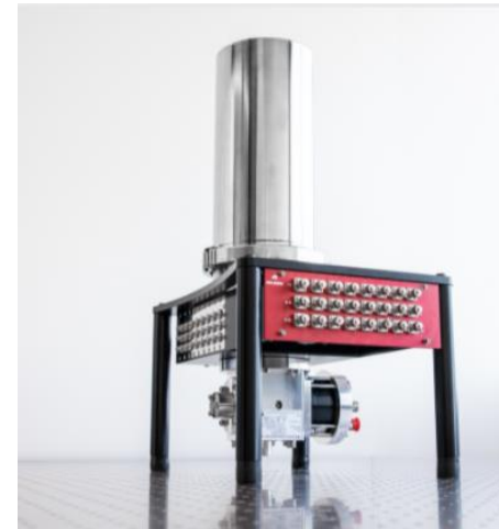
SNSPD detection mechanism and integrated measurement system
