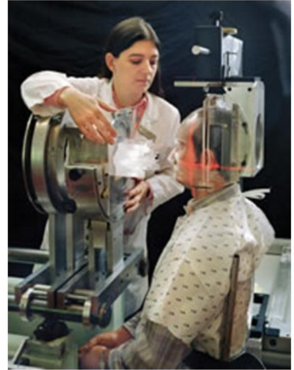
Cancer patients were treated at the Bevalac with the help of a plastic head positioner and beam compensator.
