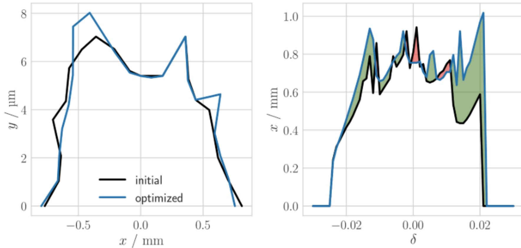
Figure 2.15: Dynamic aperture (left) and momentum aperture (right) for reference lattice (black) and optimised lattice (blue). The area of dynamic aperture is improved by 3.1 % while the area of momentum aperture is increased by 18.0 %.
