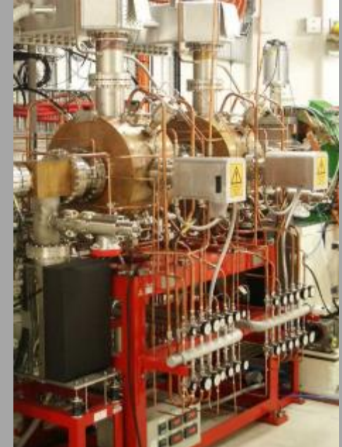
KEK/PF cavity (Toshiba) HOM damped but not at 0.8 MeV
