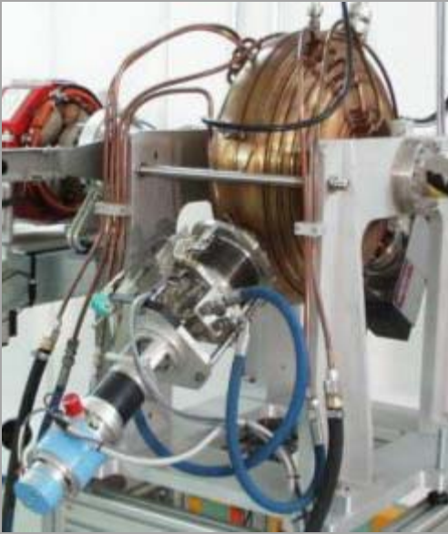
ELETTRA cavity HOM detuned but not at 0.8 MeV
