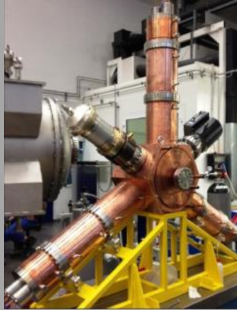
BESSY cavity (RI) HOM damped but not at 0.8 MeV
