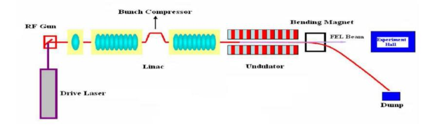
• As an alternative, electron accelerator which will drive SASE FEL, energy recovery linac (ERL) can be proposed.
