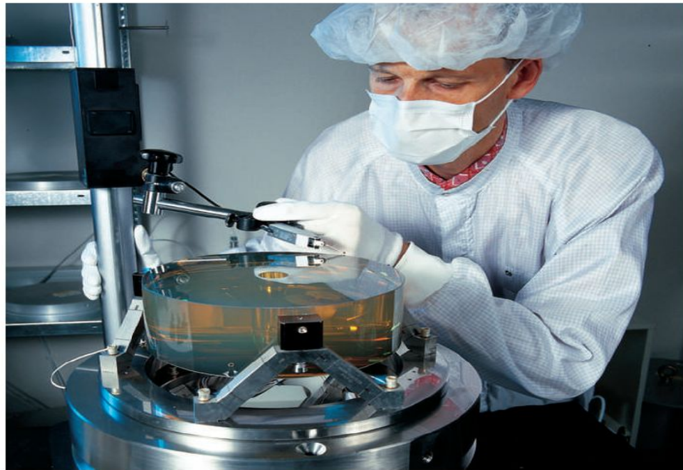
Manufacturing mirrors for EUV lithography is a huge technical challenge.
