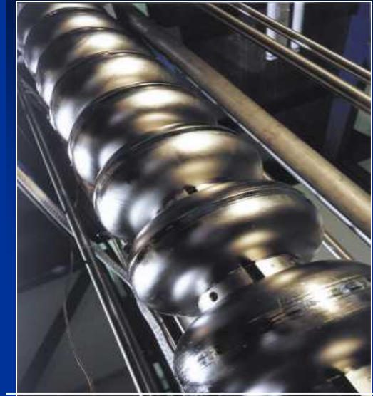
Structure of a 9-cell Nb cavity: component of linear accelerator
