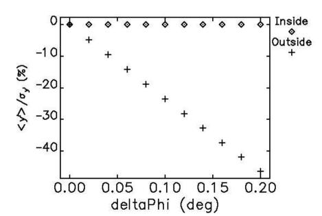
SLAC *pulsed* S-band systems have <0.1 deg rms phase jitter<sup>1</sup>
