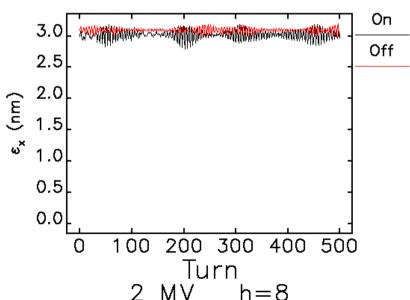
Based on simulations without synchrotron radiation, would conclude that having interior sextupoles on *at normal values* limits us to 2 MV
