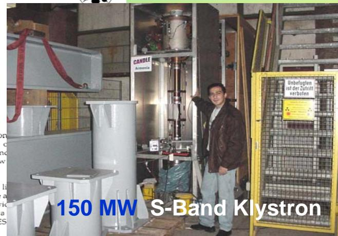
**150 MW S-Band Klystron**
